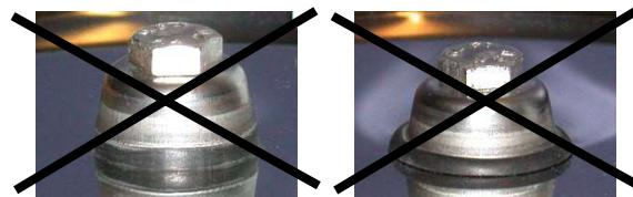
1.6 Tighten the cable gland (tightening torque of 5 N.m +/- 0.5).
