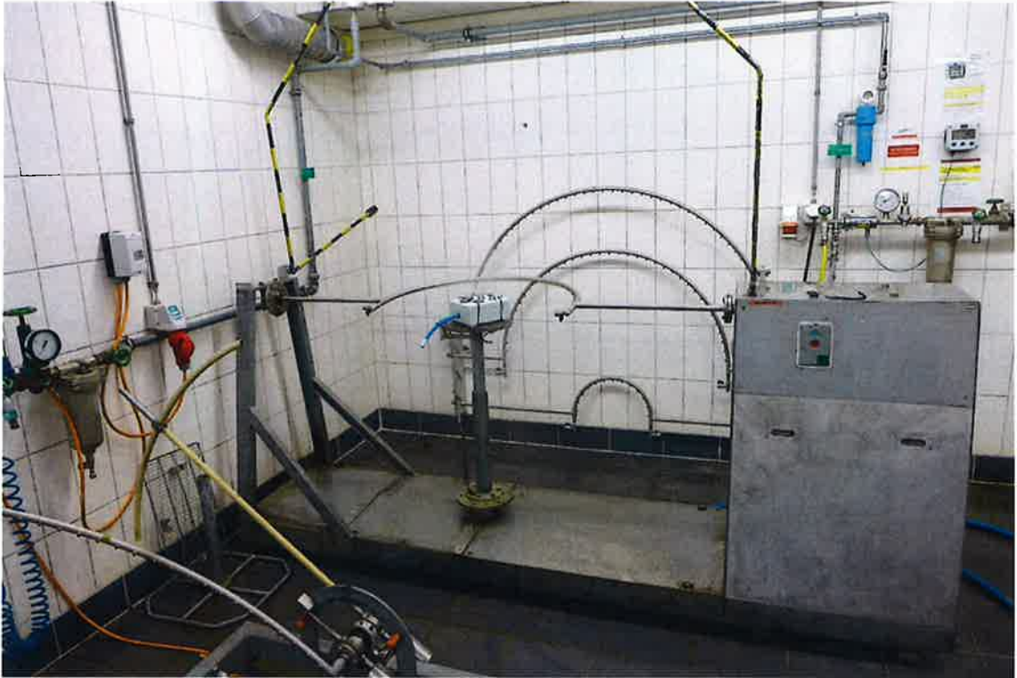
Test box during IPx4 testing:
