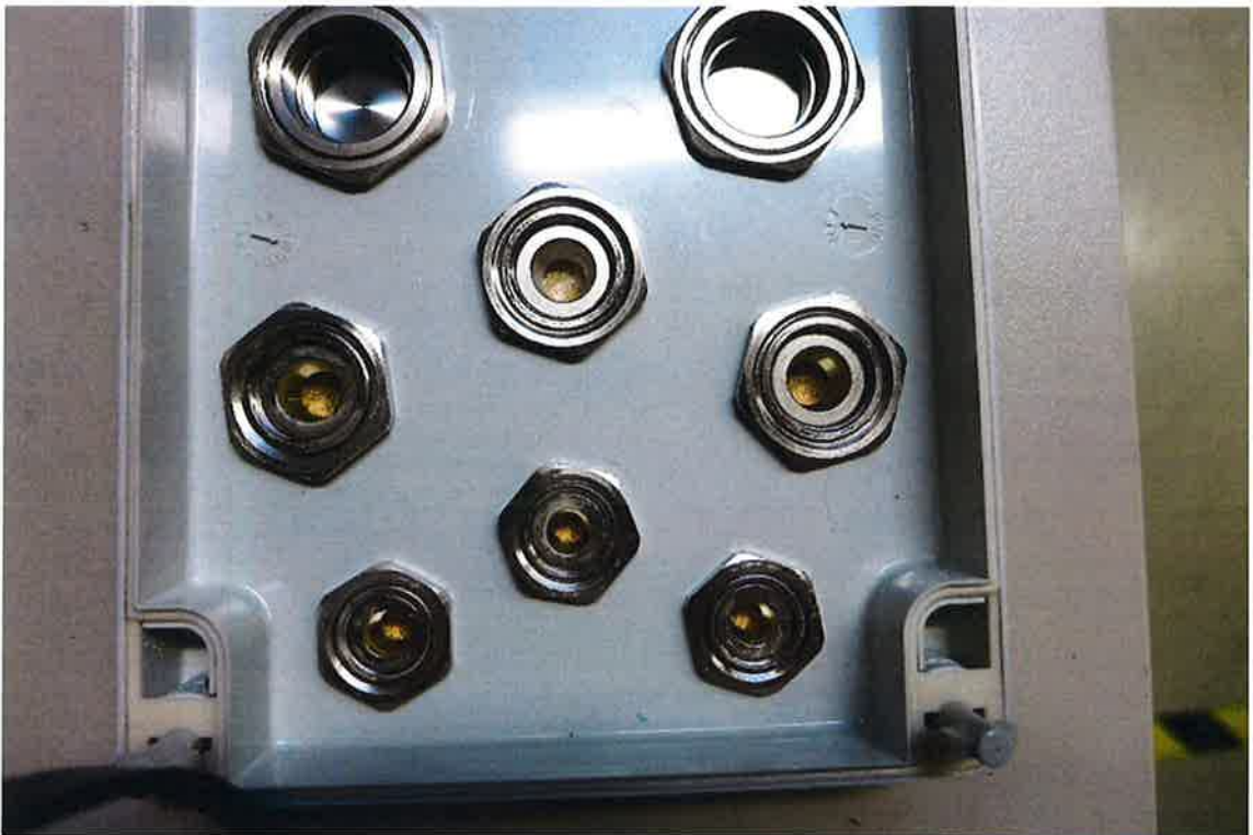
Test box after IPx4 testing. No traces of water inside the box.
