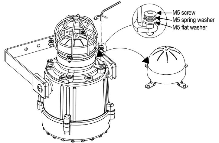
Fig. 11 Replacement of beacon lens cover
