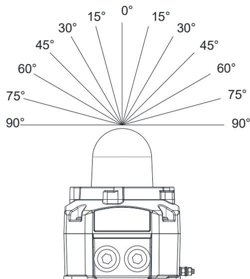
Fig. 1 – Horizontal dispersion angles for wall mounting
