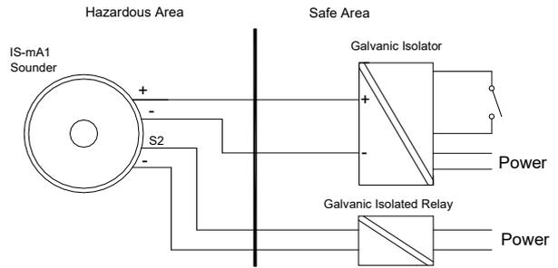
Fig 8 Multi stage alarm using galvanic isolated relays
