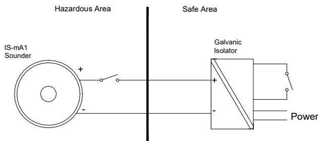
Fig 7 Single stage alarm using galvanic isolator.
