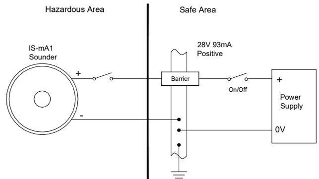
Fig 4 Single stage alarm using single channel barrier.
