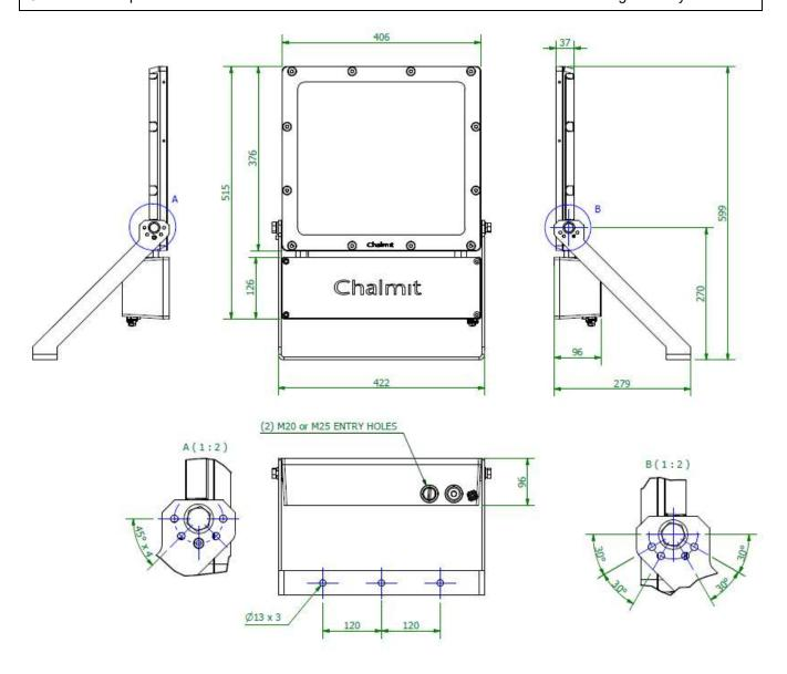
THE EVOLUTION X STIRRUP BRACKET HAS PRE-DEFINED FIXING ANGLES ALLOWING YOU TO AIM THE FLOODLIGHT AT INCREMENTS OF 30° OR 45° PLEASE REFER TO DIAGRAM ABOVE
